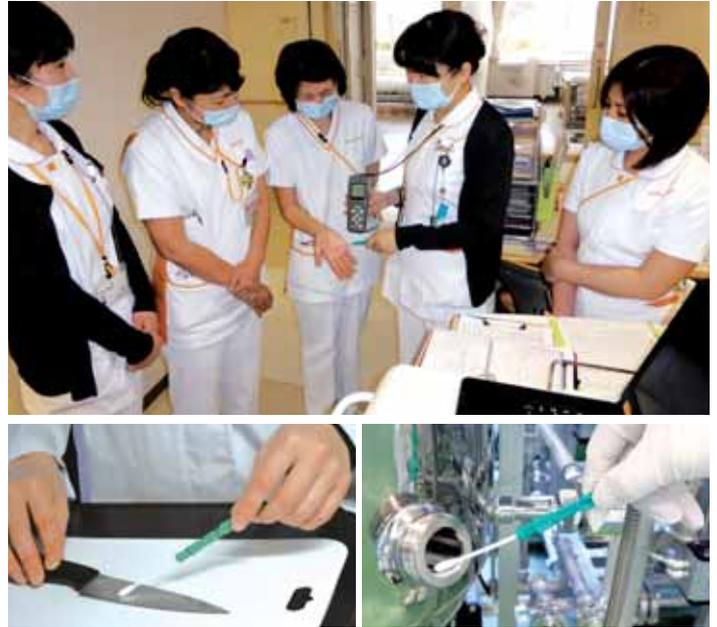
Clockwise from top: LuciPac™ A3 used to monitor hygiene in a hospital; monitoring food factory machines; wiping a knife with the special swab stick.
