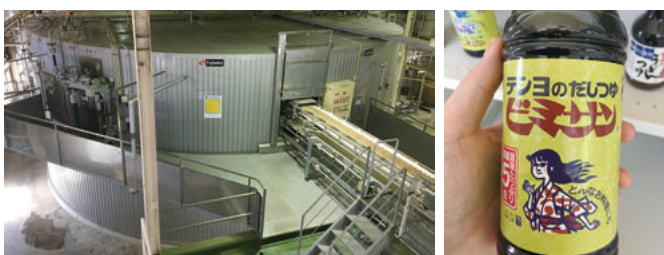
A huge 13.5m diameter disc-shaped koji production machine (left). “Bimisan” multipurpose seasoning loved in Yamanashi and nearby prefectures (right). Taken at Tenyo Co., Ltd.
